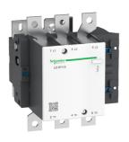
IEC contactor, TeSys F, nonreversing, 115A, 75HP at 480VAC, 3 phase, 3 pole, 3 NO, 120VAC 50/60Hz coil, open style
