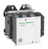
TeSys F contactor - 3P (3 NO) - AC-3 - <= 440 V 500 A - coil 220 V AC
