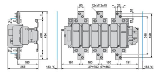
(1) Minimum distance required for coil removal.
