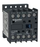
Contactor, TeSys K, 3P, AC-3/ AC-3e,440V 6A, aux. 1NO, 220...230V AC coil, screw clamp terminals
