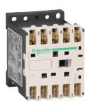
TeSys K contactor , 3P , AC-3 <= 440 V 9 A , 1 NO aux. , 230...240 V AC coil
