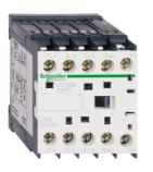
TeSys K contactor , 3P , AC-3 <= 440 V 16 A , 1 NC aux. , 24 V AC coil
