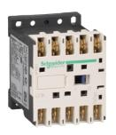
TeSys K contactor , 3P , AC-3 <= 440 V 16 A , 1 NC aux. , 230...240 V AC coil
