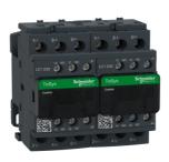
Reversing Contactor, TeSys Deca, 3P(3NO), AC-3, <=440V, 32A, 115V AC 50/60Hz coil, screw clamp terminals
