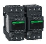
Reversing Contactor, TeSys Deca, 3P(3NO), AC-3, <=440V, 40A, 400V AC 50/60Hz coil, screw clamp terminals
