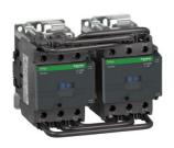
Reversing Contactor, TeSys Deca, 3P(3NO), AC-3/AC-3e, <=440V 80A, 110V AC 50/60Hz coil, screw clamp terminals
