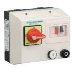
Enclosed DOL starter, TeSys LG, 1-1.6A, 220/230V AC coil, including 1 LC1K, GV2ME, rotary isolation switch ,2 pushbuttons
