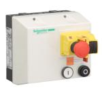
Enclosed DOL starter, TeSys LG, 0.63-1A,380/400V AC coil, including 1 LC1K, GV2ME with emergency stop,2 pushbuttons
