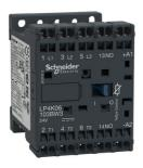
Contactor, TeSys K, 3P, AC-3/ AC-3e, 440V, 12A, 1NO aux, 24V DC low consumption coil, spring terminal
