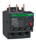
Thermal overload relay, TeSys Deca, 690VAC, 9 to 13A, 1NO+1NC, class 10A, for D12…D38 unbalanced loads
