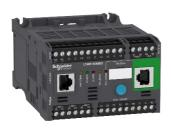
Motor Management, TeSys T, motor controller, Modbus, 6 logic inputs, 3 logic outputs, 5 to 100A, 24VDC
