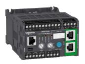
Motor controller, TeSys T, Motor Management, Ethernet/IP, Modbus/ TCP, 6 inputs, 3 logic outputs, 1.35A to 27A, 24VDC
