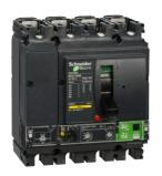
Circuit breaker, ComPact NSX250B, 25kA/415VAC, MicroLogic 4.2AB Vigi trip unit, 240A, 4 poles 4d
