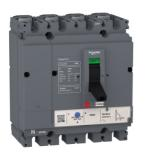
circuit breaker EasyPact CVS160F, 36kA at 415VAC, 100A rating thermal magnetic TM-D trip unit, 4P 3d
