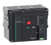
Switch disconnector, MasterPact MTZ2 16NA, 1600A, 88kA/690VAC 50/60Hz (Icm), 3P, drawout
