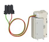
MN opening undervoltage release, MasterPact MTZ2/MTZ3 drawout, standard, 200/250VAC 50/60Hz, 200/250VDC
