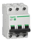
Miniature circuit breaker (MCB), Multi9 C60SP, 3P, 8A, C curve, 10kA (UL1077), 10kA (IEC/EN 60947-2)
