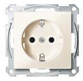
Socket-outlet, Merten System M, mechanism with fixing frame, 2P + E, 16A, Schuko, screwless terminals, glossy, white
