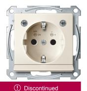
Socket-outlet, Merten System M, mechanism with fixing frame, 2P + E, 16A, Schuko, screwless terminals, glossy, white
