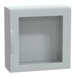
Floor standing polyester enclosure, Thalassa PLA, glazed door, completely sealed, 750x750x320mm, IP65, IK08
