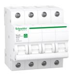
Miniature circuit breaker (MCB), Resi9, 4P, 10A, C curve, 3000A (IEC/EN 60898-1)
