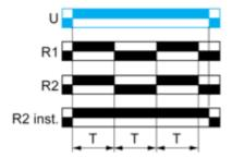
Function Dit: Symmetrical Flashing Relay (Starting Pulse On) & With Pause / Summation Control
