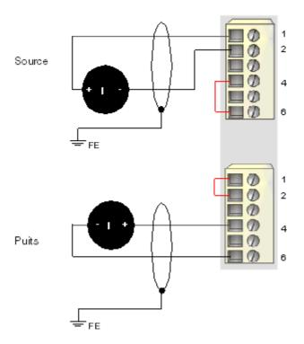
2 isolated analog actuators, external 24 VDC power supply
