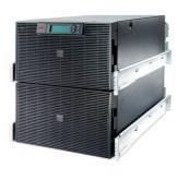
APC Smart-UPS RT 15kVA, 230/400V, LCD, rackmount, 12U, 2x IEC Jumpers & 8x IEC 60320 C19 outlets
