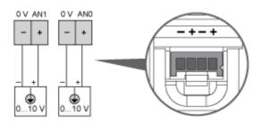
The (-) poles are connected internally.
