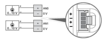
The (-) poles are connected internally.
