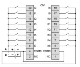
The COM0 terminals are connected internally
