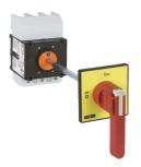
Switch disconnector, TeSys Control, for ON/emergency stop, 175A,4 screws fixing, for mounting at back of an enclosure
