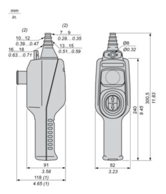
(1) With trigger action latching Ø 30 mm / 1.18 in. Emergency stop. (2) Internal Ø
