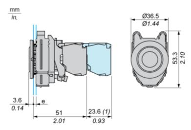
$\boldsymbol{e}$  : clamping thickness: 1 to 6 mm / 0.04 to 0.24 in. (1) : Additional row of contacts
