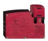
Safety switch, Telemecanique Safety switches XCS, plastic XCSTE, 2 NC, slow break, 1entry tapped M16, 24 V
