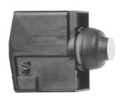
Push button for control circuit, Harmony XAC, plastic, black, booted, 0...15V DC, 1 NO + 1 NC at start of travel, 1 NO at end of travel
