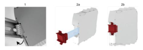
1 : Mount controller CPU and modules on rail.
