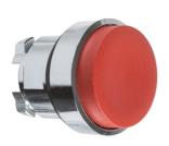
Head for illuminated push button, Harmony XB4, metal, red projecting, 22mm, push-push, unmarked
