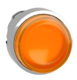
Head for illuminated push button, Harmony XB4, metal, orange projecting, 22mm, push push, universal LED, unmarked
