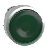
Head for illuminated push button, Harmony XB4, metal, green flush, 22mm, universal LED, spring return, plan lens
