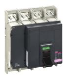
circuit breaker basic frame. ComPact NS 630bL. 150 kA at 415 VAC. 630 A. fixed. manually operated. without trip unit. 4 P
