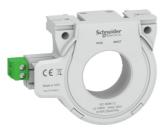
closed toroid A type. for VigiPacT and Vigilhom. TA30. inner diameter 30 mm. rated current 65 A
