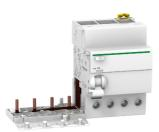
Vigi iC60 - earth leakage add-on block - 4P - 40A - 300mA - AC type
