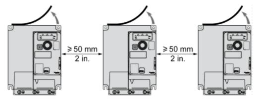
For Operation at Ambient Temperature Above 50 °C (122 °F)
