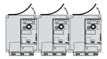
Mounting Type C: Individual, Ventilation Cover Removed
