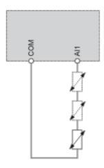
It is possible to connect either 1 or 3 sensors on terminals Al1.
