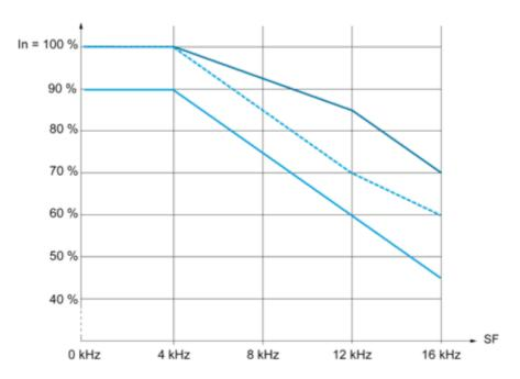
40 °C (104 °F) - Mounting type A, B and C 50 °C (122 °F) - Mounting type A, B and C 60 °C (140 °F) - Mounting type B and C
