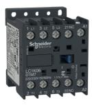
TeSys K contactor - 3P - AC-3 <= 440 V 9 A - 1 NC aux. - 380...400 V AC coil
