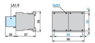
Reversing Contactors LC2 K, LP2 K, LP5 K: Mounting on Rail AM1 DP200 or AM1 DE200 (35 mm)
