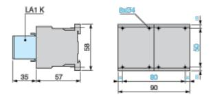
Reversing Contactors LC2 K, LP2 K, LP5 K: Mounting on Rail AM1 DP200 or AM1 DE200 (35 mm)
