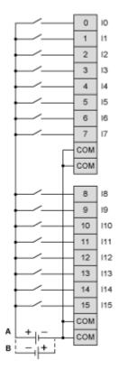
The 4 COM terminals are connected internally
